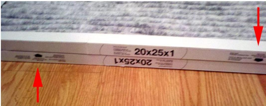
With the filters lined up, tape one of the short (20") edges of the filters to create a hinge between the two filters, as shown below.
