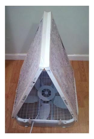
Use a strip of tape to secure each end of the filers to the fan. **NOTE: It is better if there are some small leaks, so don't worry about getting it airtight.**
