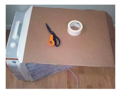
Flip the cardboard up using the taped edge as a hinge and cut along the traced lines with scissors. Then tape the cut edges of the cardboard to the filters.
